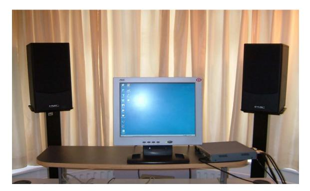
I generally suggest the monitors be placed at an angle of 60 degrees to the listener and the whole listening 'stage' to form an equilateral triangle. This provides the optimum angle to fully image the entire stereo field.
